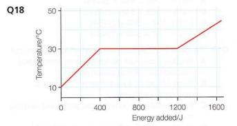
The heating curve for 10g of a substance is given above. How much energy would be required to melt completely 40g of the substance that is initially at 10°C ?
